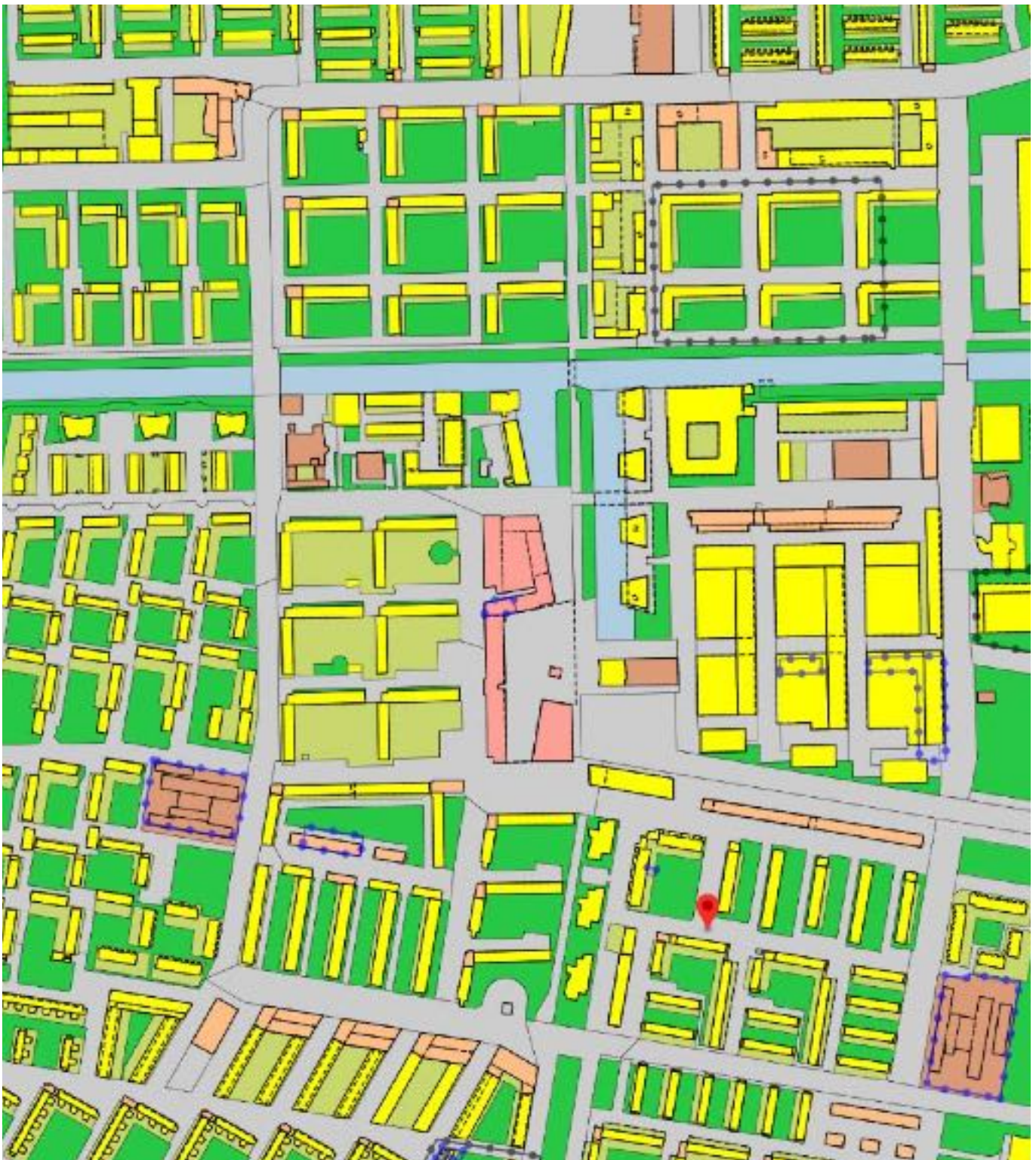
figure 2.4. a more modern and smaller scale example is this zoning plan for the neighbourhood Geuzenveld in Amsterdam. This plan shows which functions can take place in which areas. Yellow shows housing, grey is traffic, brown areas have a societal function and pink are areas for shops and trade (Gemeente Amsterdam, 2010)
