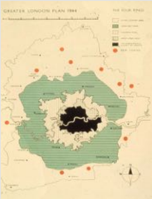
figure 3.23. The Greater London Plan of Abercrombie introduced four rings, an inner city ring, a suburban ring, a green belt and an outer country ring around the city (Abercrombie, 1944)
